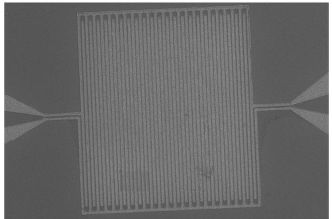
*Figure 1: Scanning Electron Microscope image of a typical SSPD made on NbN ultrathin films : surface 10x10  $\mu\text{m}^2$ , the wire is 70 nm wide and 50  $\mu\text{m}$  long.*
